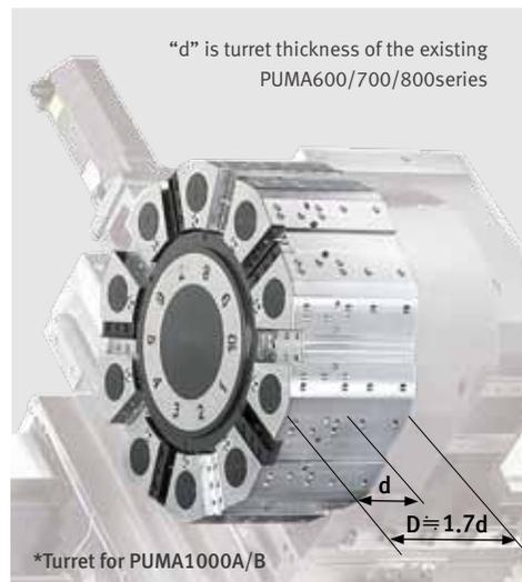
Turret indexing is possible with  $\varnothing$ 100 x L1000mm ( $\varnothing$ 3.94 x 39.4") sized long boring bar in its turret.
